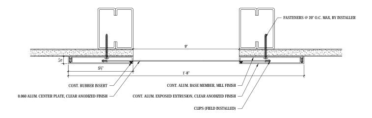
NOTE: 1 HOUR CONSTRUCTION INDICATED 2 LAYERS OF GYPSUM BOARD FOR 2 HOUR CONSTRUCTION
